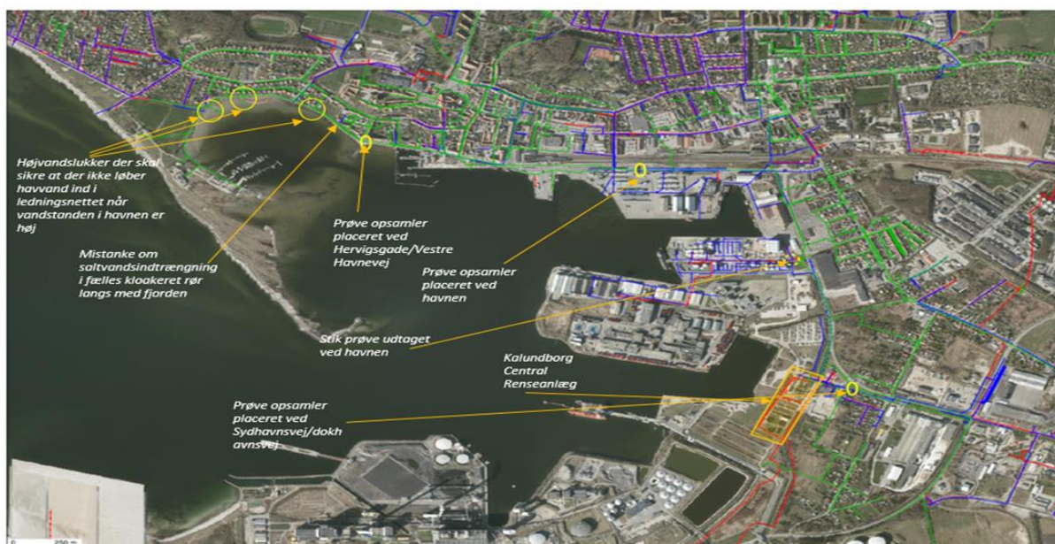
Figure 4. Wastewater collection system of Kalundborg with possible bromide sources
