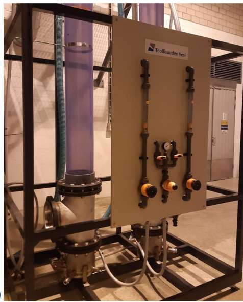
a) bottom nozzles, b) flow and air pressure control and connections for washwater and air
