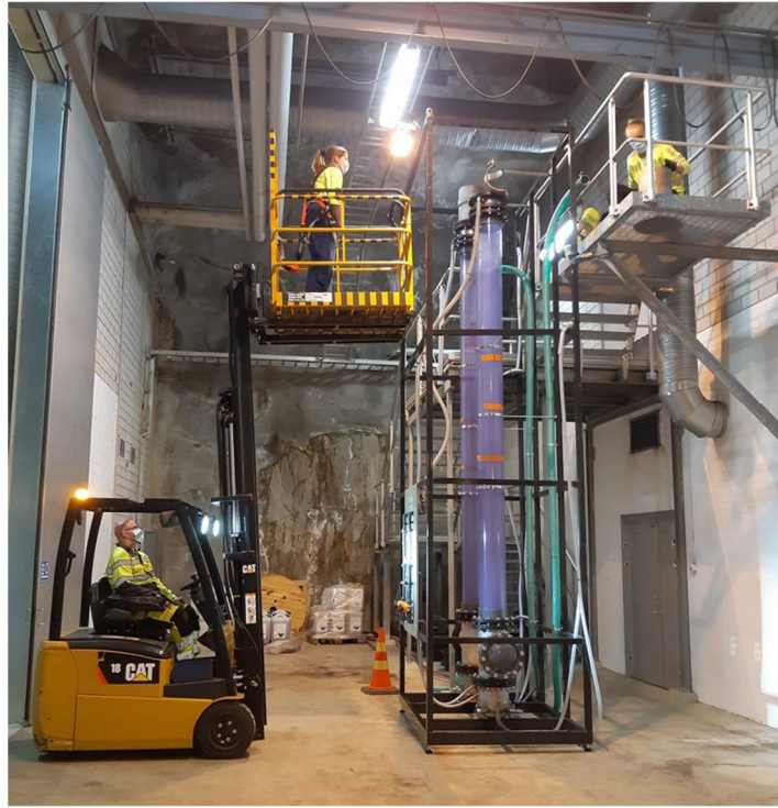
a) The pilot on site before the addition of GAC, b) changing of gaskets
