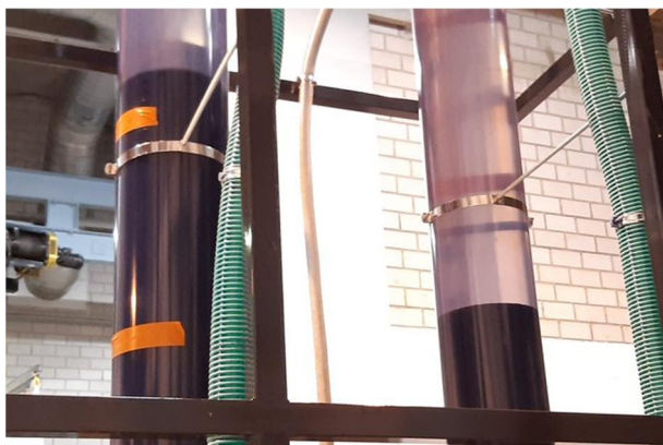
Figure 5. The top of filter beds during washing. Virgin GAC on the left. The virgin GAC filter bed expansion is much higher and the surface appears fuzzy due to small filter particles moving.
