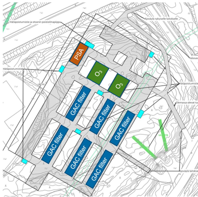
Figure 4. Process lay-out for reservation in underground city zoning 4 . The light blue rectangles are emergency exits with structures above ground.
