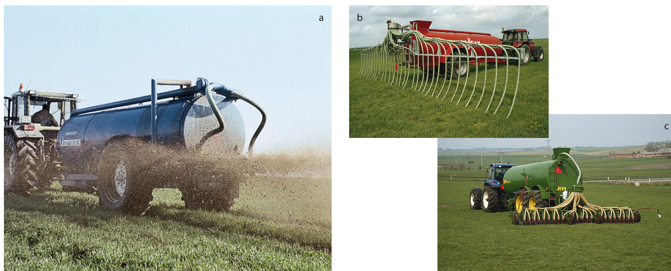
Figure 3. Technological innovations for manure spreading on agricultural land: a) broadspreading (older technology), b) trailing hoses (newer technology) and c) injection (modern technology).
