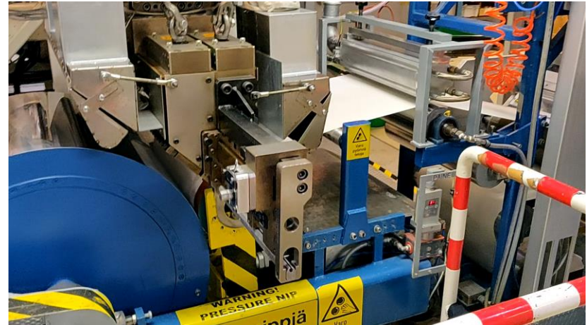
Pilot scale extrusion coater at Tampere University
