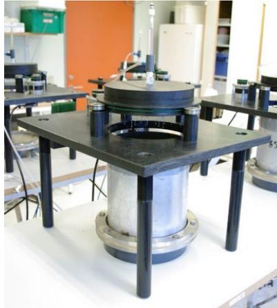
Figure 5. Soil column ready in the leaching set-up
