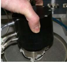
3. Adjust the pressure to approximately -5 cm using the pressure controller
