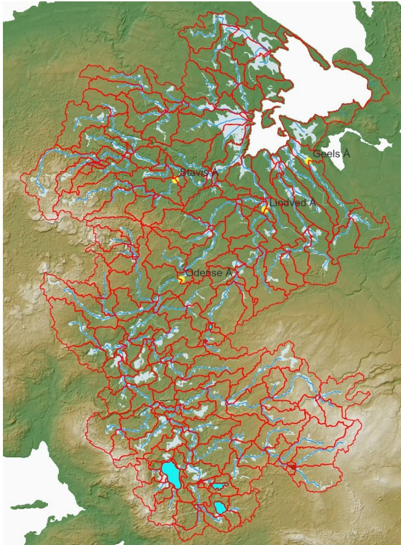
Figure 2. Watershed, subbasins, lakes, and streams delineated by SWAT+ with floodplain delineation (light shaded areas). The gauging stations are indicated by yellow points.
