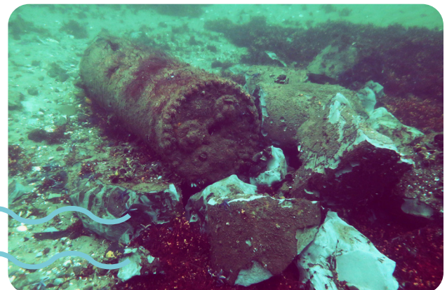
Corroded munition on the Baltic seabed. © GEOMAR
