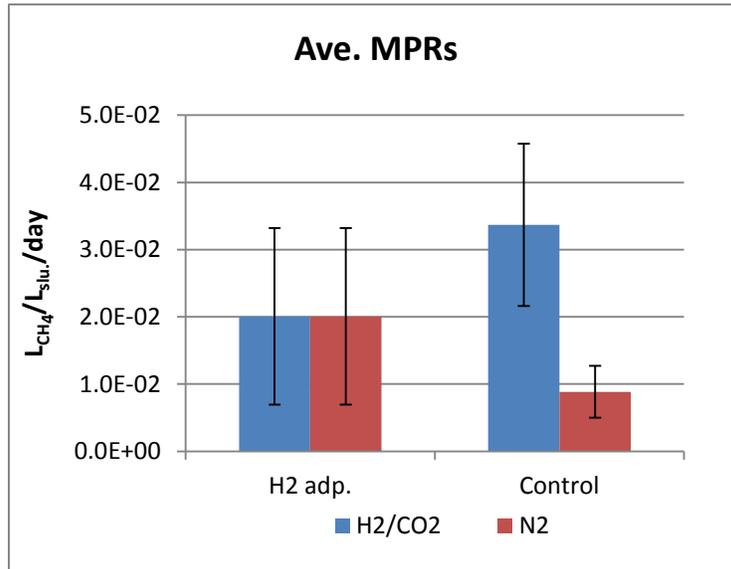
**Figure 30: Methane production rate** in liter methane produced per liter reactor slurry per day. The slurry from H<sub>2</sub> adapted and control laboratory scale reactors, 1mL slurry diluted in 5mL saline water with a headspace of H<sub>2</sub>/CO<sub>2</sub> (80:20) or N<sub>2</sub>. There was no significant difference between any of the samples, tested with a Students t-test. Standard deviations are indicated by error bars.
