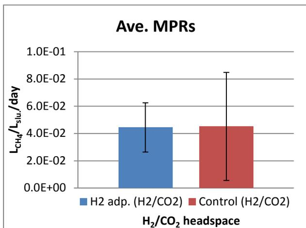
**Table 18: Methane production rates**, liter methane produced per liter reactor slurry per day, H<sub>2</sub> adapted and control replicas with H<sub>2</sub>/CO<sub>2</sub>. The rates were calculated from the slope of the linear regression of the methane production over time. Standard deviations are indicated by error bars
