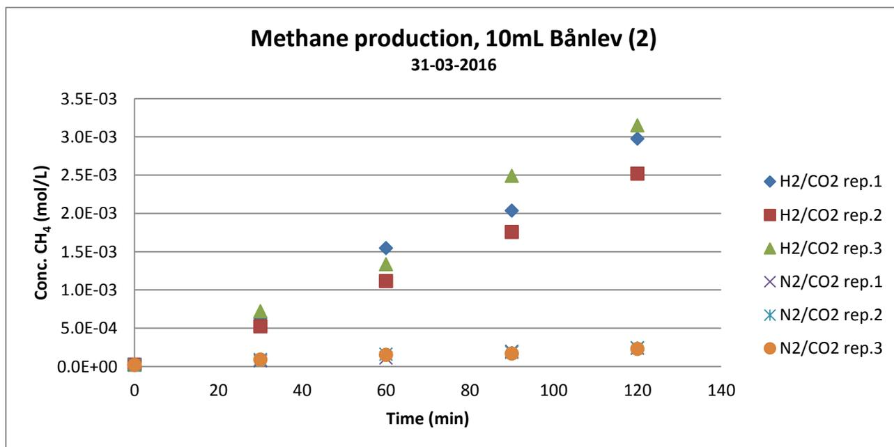
**Figure 17: Methane production with slurry from Bånlev Biogas, 10mL undiluted slurry with a headspace of either H<sub>2</sub>/CO<sub>2</sub> or N<sub>2</sub>/CO<sub>2</sub> in the ratio 80:20.** Linear regressions, H<sub>2</sub>/CO<sub>2</sub> headspace samples:  $y(\text{rep.1}) = 2.44\text{E-}05x - 2.05\text{E-}05$  ( $R^2 = 0.992$ ),  $y(\text{rep.2}) =$
