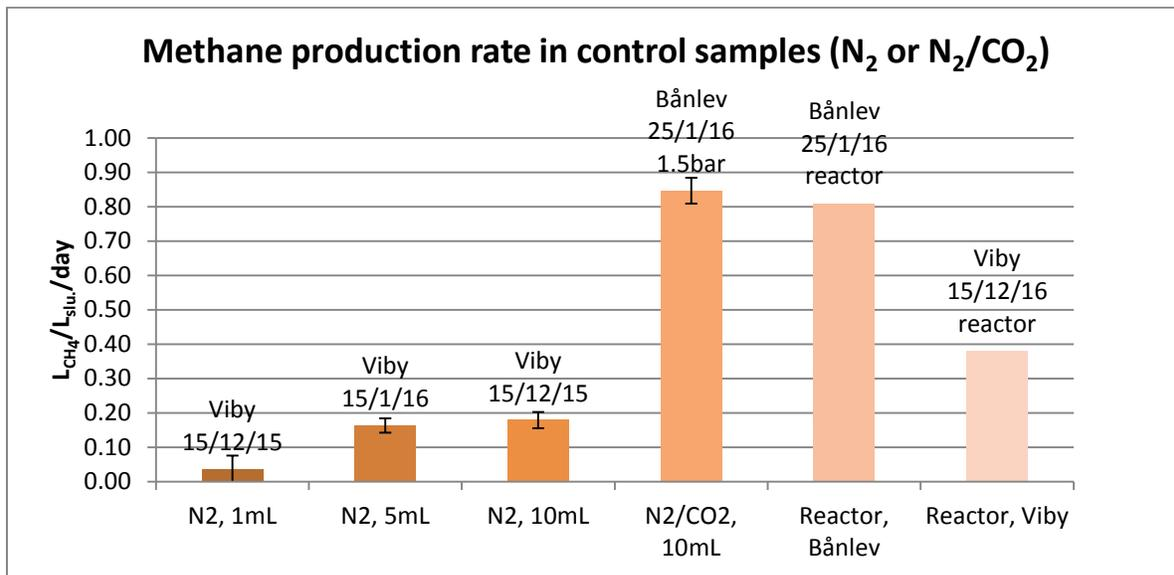
**Figure 16: Methane production rate** in liter methane per liter slurry per day, displaying the average rates of control samples. Slurry from Viby WWTP, 1mL (1:10 dilution) and 5mL (1:1 dilution), and undiluted (15/12/15) with N<sub>2</sub> headspace is shown. Undiluted slurry, 10mL, from Bånlev Biogas with N<sub>2</sub>/CO<sub>2</sub> headspace is also shown. The reactor rates were calculated with data from reactor monitoring programs at site. Standard deviations are indicated by error bars.
