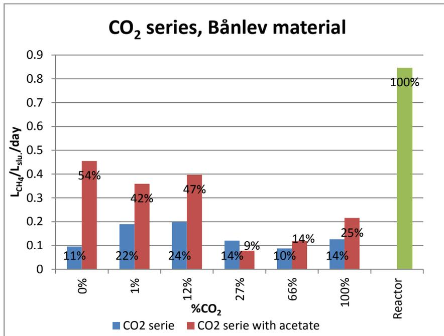
**Figure 28:** Methane production rate in liter methane produced per liter reactor slurry per day. 10mL slurry from the anaerobic digester at Bånlev Biogas was used with headspace N<sub>2</sub>/CO<sub>2</sub> and different CO<sub>2</sub> concentration. Acetate was added in one of the series. The methane production rate of the reactor at sampling time is shown. The rate in percentage of the reactor rate is indicated.
