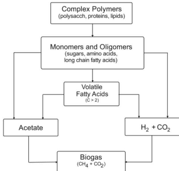
Figure 1: Schematic presentation of stages in the anaerobic digestion. (Weiland 2010)
