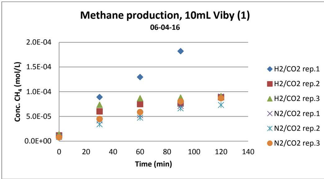
Figure 19: Methane production with slurry from Viiby WWTP, 10mL undiluted slurry with a headspace of either H<sub>2</sub>/CO<sub>2</sub> or N<sub>2</sub>/CO<sub>2</sub> in the ratio 80:20.
