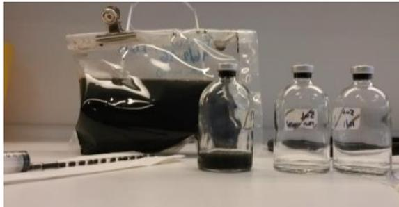
**Figure 3: Slurry in plastic bag, sealed serum bottle with slurry**
