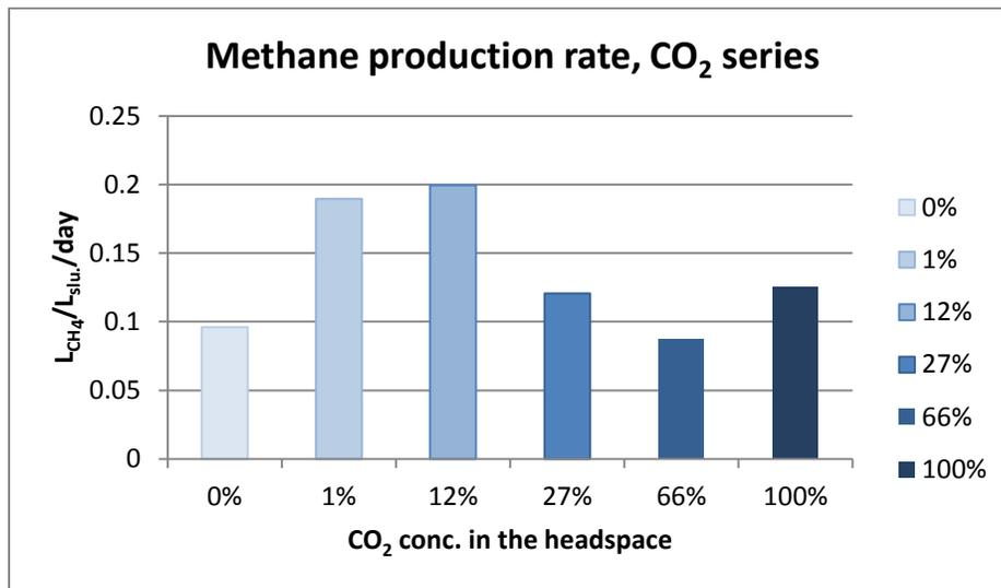
**Figure 25: Methane production rate** in liter methane produced per liter slurry per day. 10mL slurry from the anaerobic digester at Bånlev was used with headspace of N<sub>2</sub>/CO<sub>2</sub> with different CO<sub>2</sub> concentration. MPR was calculated from the slope of the linear regression of methane production over time.
