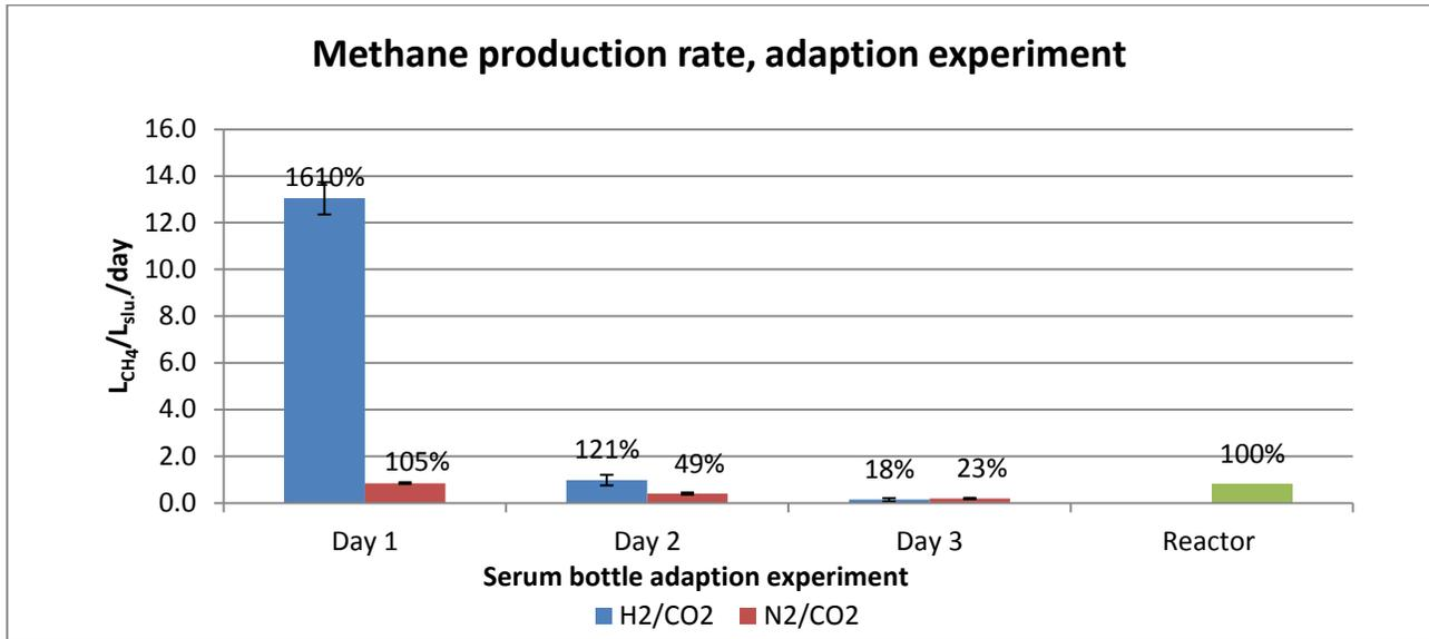
**Figure 34: Methane production rate** in liter methane produced per liter slurry per day. The same serum bottles and slurry was tested day 1, 2 and 3. The headspace was either H<sub>2</sub>/CO<sub>2</sub> or N<sub>2</sub>/CO<sub>2</sub> (80/20). Ave. MPR in percentage of the reactor rate indicated above the column. Standard deviations are indicated by error bars.
