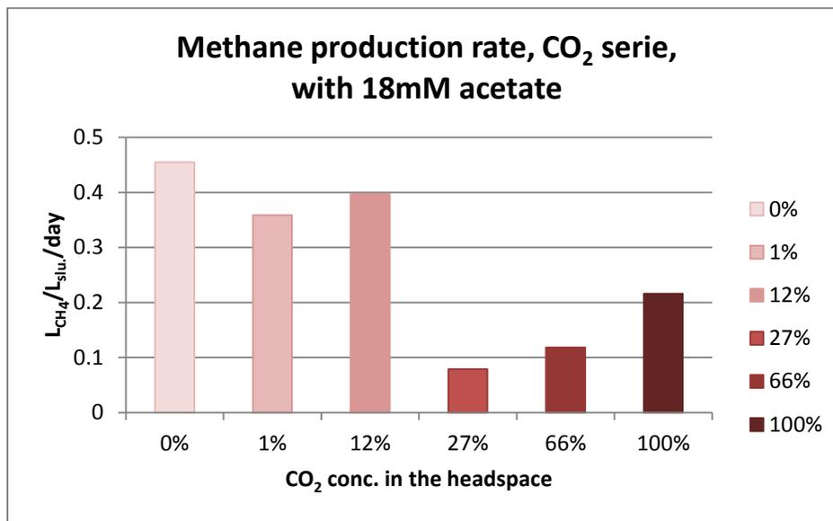
**Figure 27:** Methane production rate in liter methane produced per liter reactor slurry per day. The slurry was from Åby WWTP, 10mL slurry with 18mM added acetate and with a headspace of N<sub>2</sub>/CO<sub>2</sub> with different CO<sub>2</sub> concentration.
