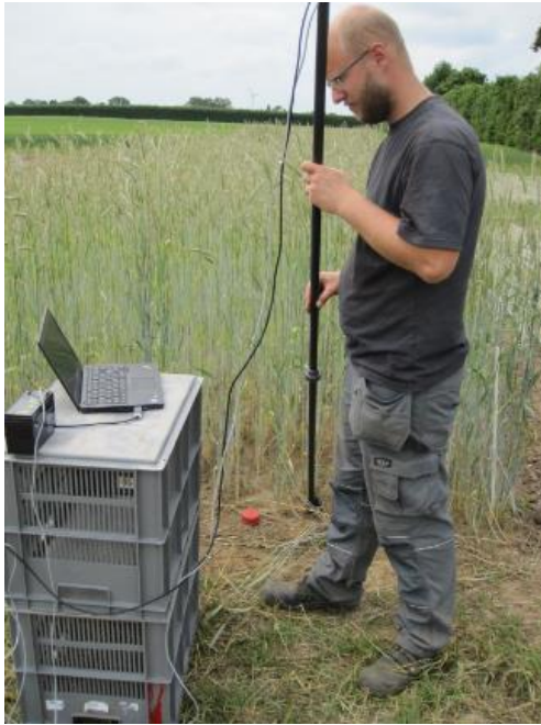
Non-destructive root registration in minirhizotrons
