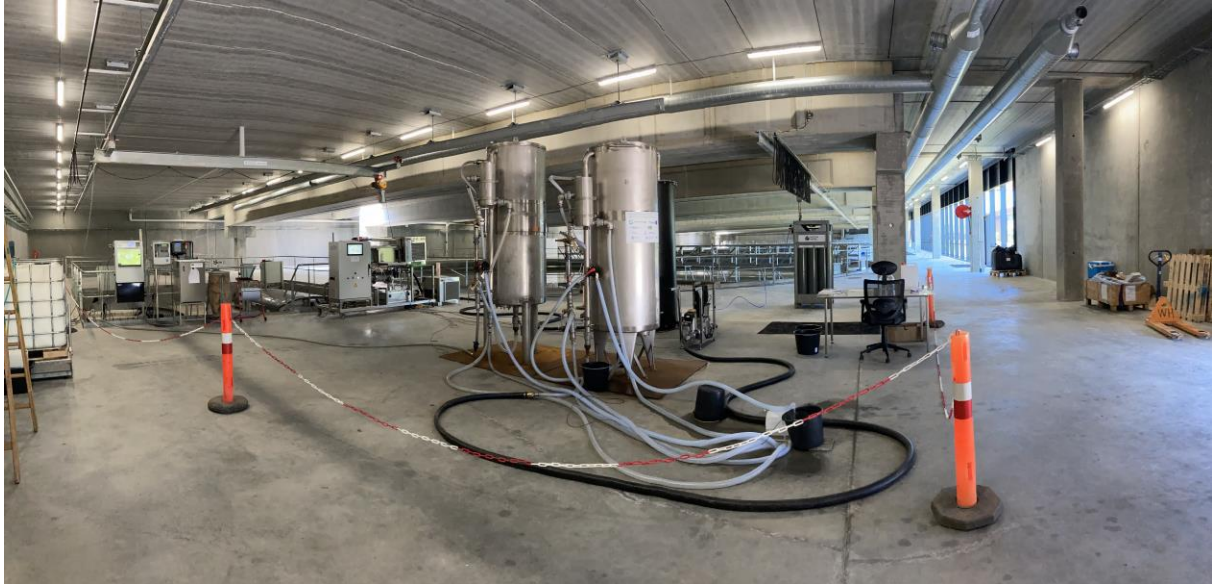
SI-Figure 2. GAC pilot plant filters with samplings points at WWTP in Hillerød.
