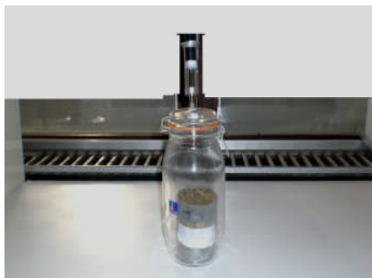
Figure 2. Gas sampling from an air tight jar with soil core inside
