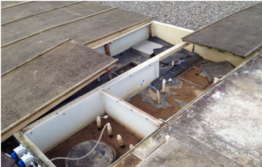
Figure 2: Picture of pilot scale denitrifying bioreactor test facility (10*4*1.5 m) containing aquifer and woodchip cells. It has the capacity to inject contaminated water, remediate this water and investigate removal in a holistic way.
