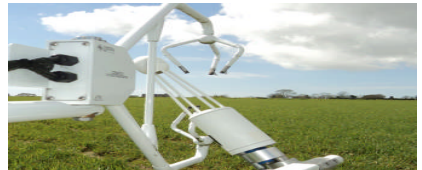
Figure 1. Components of the eddy covariance systems consisting of a 3-D sonic anemometer and fast response CO 2 infra-red gas analyser.
