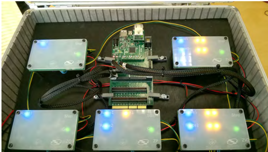
Figure 11: The distributed Hardware in the Loop prototype
