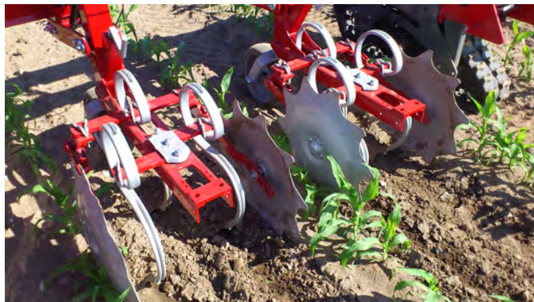
Figure 14: Two different row cleaning implements mounted on Robotti and tilling the soil.
